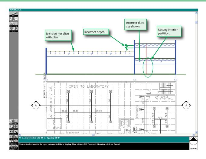
In this solution, there are multiple errors. As drawn, the largest duct on the second floor will not fit between the lights and the joists above. On the first floor, there is a duct that is incorrectly sized and an interior partition cut by the section line is missing.
