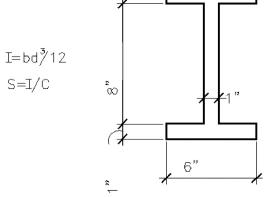
**5.** What is the section modulus for the geometric section illustrated above?
