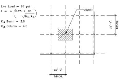
**6.** When considering permitted live load reductions for the column shown above, what is the live load for the floor supported by the column?
