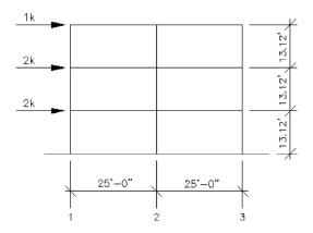
**21.** For the rigid frame structure shown, the approximate horizontal shear at the base of column 2 (assuming all column stiffnesses are equal) is
